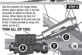
Another view showing ties on the engine. Wrap zip ties in 2 places on engine (A-B) and use one of the 3 holes provide to wrap 3rd zip tie (C)
